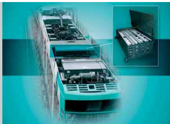
Left: Test vehicle AutoTram®. First employment of the „DockingPrinciple“. Right: An important element of the new propulsion system is a Bombardier* MITRAC® Energy Safer.
