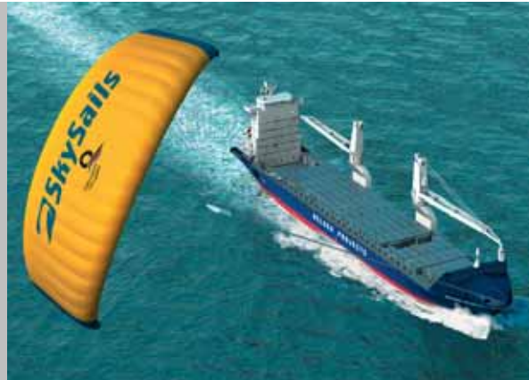
Left: SkySails towing kite system on the coastal vessel "MS Beaufort". Right: The illustration shows the system installed on a cargo ship.
